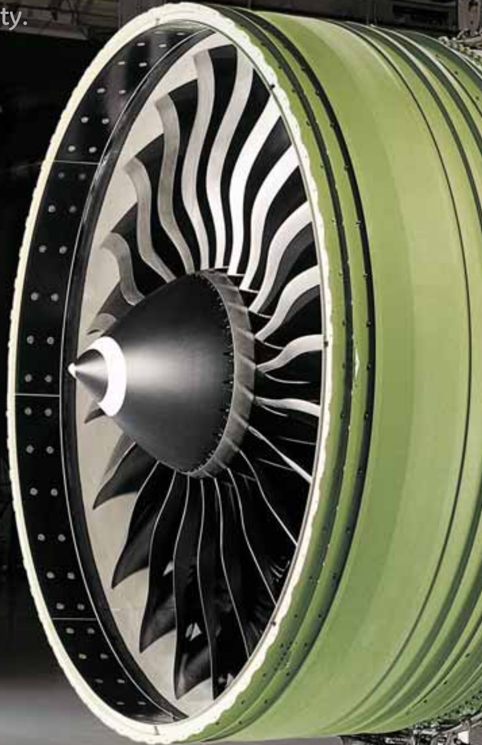
GE90-115B engine being prepared for test. The engine is assembled at GE's Durham, North Carolina and Peebles, Ohio facilities
